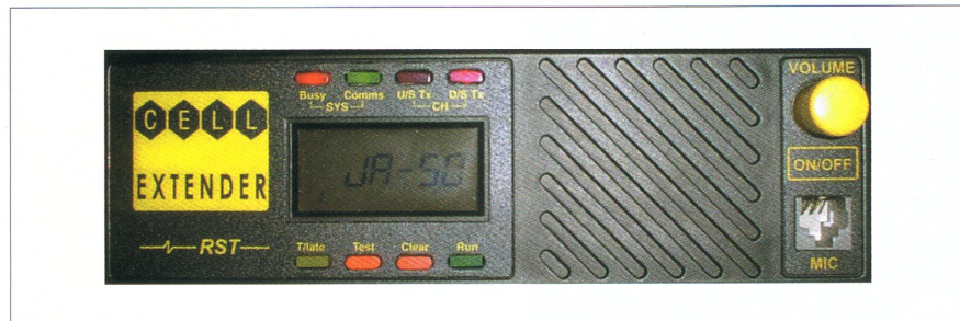
Figure 3: Photograph of the Jammer Control Module. Its built-in intelligence will ensure that when the prime Control Channel would move (eg, when the system switches to a secondary Control Channel) the Jammer follows that move. And when for instance, the adjacent (referred CONT) site is off the air (for whatever reasons), it should stop jamming altogether.
